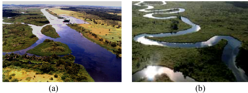
Figure 2. Channelized Kissimmee River (a) versus restored system (b) (from Wikimedia Commons (a), http://commons.wikimedia.org/wiki/File:Kissimmee_River_canal_section.jpg , and South Florida Water Management District (b), http://www.sfwmd.gov/portal/page/portal/pg_grp_sfwmd_watershed/pg_sfwmd_watershed_kissimmee )
