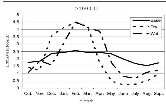
Figure 1. Monthly generation above 1000 ft range under different climatic conditions (No-Storage Approach)
